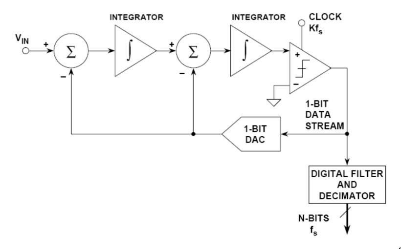
Noise reduction properties of Sigma-Delta ADCs
