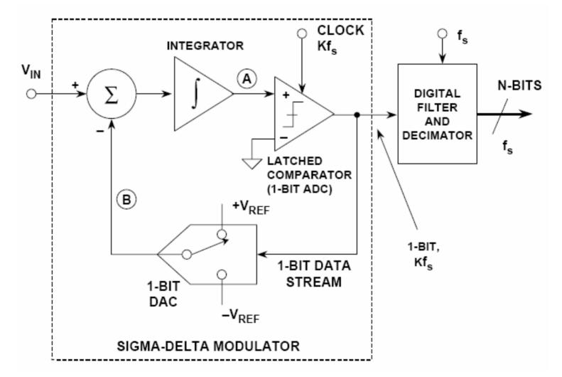
Linearized model of Sigma-Delta ADC
