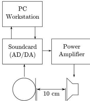
**Fig. 3:** Measurement setup used for the identification of the loudspeaker model.
