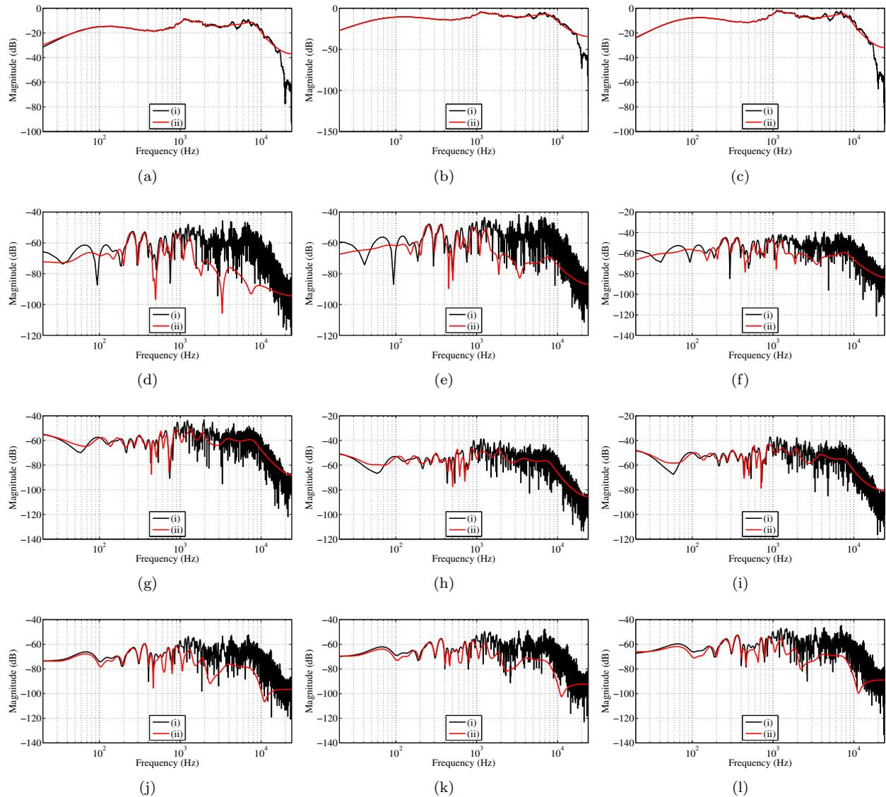
**Fig. 8:** Estimated (i) and modeled (ii) magnitude frequency responses using 40th order common-pole parallel filters. (a)-(c) Chebyshev polynomial  $C_1(x)$  for RMS input voltage 3, 5, and 7 V. (d)-(f) Chebyshev polynomial  $C_2(x)$  for RMS input voltage 3, 5, and 7 V. (g)-(i) Chebyshev polynomial  $C_3(x)$  for RMS input voltage 3, 5, and 7 V. (j)-(l) Chebyshev polynomial  $C_4(x)$  for RMS input voltage 3, 5, and 7 V. Note different scales on the  $y$  axis.
