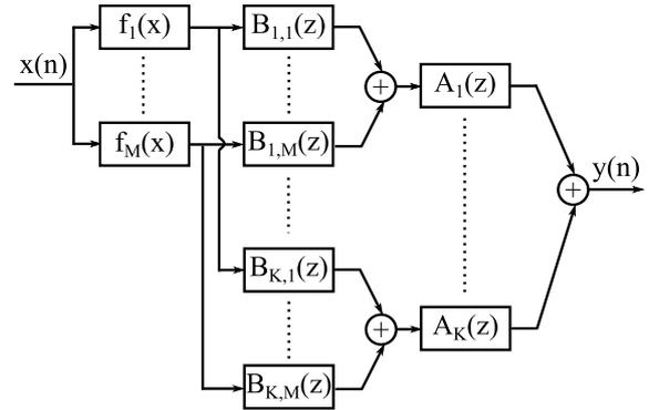
**Fig. 2:** Proposed efficient model implementation based on common-pole parallel filters.
