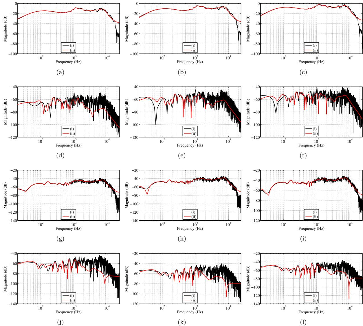
**Fig. 7:** Estimated (i) and modeled (ii) magnitude frequency responses using 40th order common-pole parallel filters. (a)-(c) Legendre polynomial  $L_1(x)$  for RMS input voltage 3, 5, and 7 V. (d)-(f) Legendre polynomial  $L_2(x)$  for RMS input voltage 3, 5, and 7 V. (g)-(i) Legendre polynomial  $L_3(x)$  for RMS input voltage 3, 5, and 7 V. (j)-(l) Legendre polynomial  $L_4(x)$  for RMS input voltage 3, 5, and 7 V. Note different scales on the  $y$  axis.
