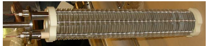
Figure 1. Photograph of an LHC ionization chamber with the cylindrical insulating cover removed [2]. Notice the stack of aluminum electrodes and the ceramic insulation at both ends.
