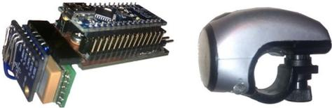
Fig. 1. The data collection system, built in the case of a bicycle lamp
