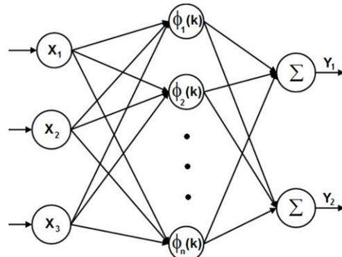
Figure 2. The radial basis function neural network structure
