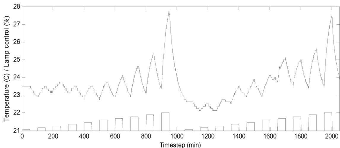
Figure 3. Internal temperature and lamp control signal recorded in the small scale experimental greenhouse
