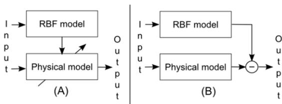
Figure 1. Possible hybrid modeling implementations: A) serial; B) parallel;
