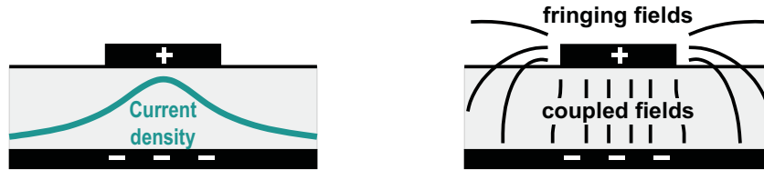
Figure 15. Ground Plane Acting as a Single Return Trace
