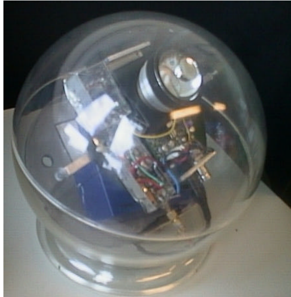
Figure 7. Breadboard model of the proposed under-water inspection and mapping device.
