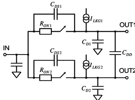
Figure 4. Model of an analog switch
