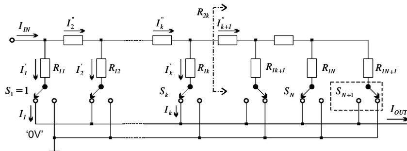
Figure 3. Inverse ladder as cascaded current dividers
