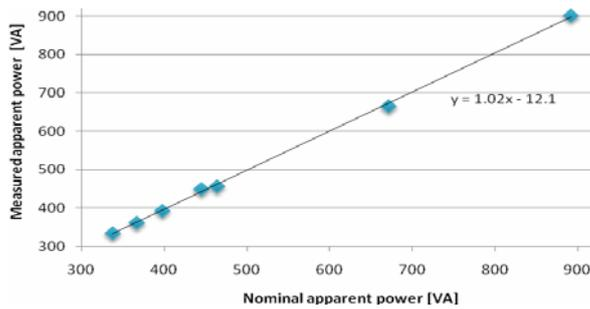
Table I Experimental results attained in the measurement of apparent power.
