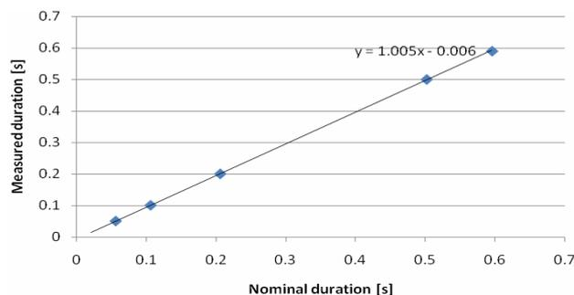
Table II Experimental results attained in the measurements of sag duration.
