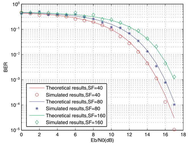
Fig. 5. BER performance of the CS-DCSK modulation scheme over AWGN channel. Solid lines show the BER performance calculated from the analytical expression, while the values marked by circles, asterisks and diamonds give the results of computer simulations.
