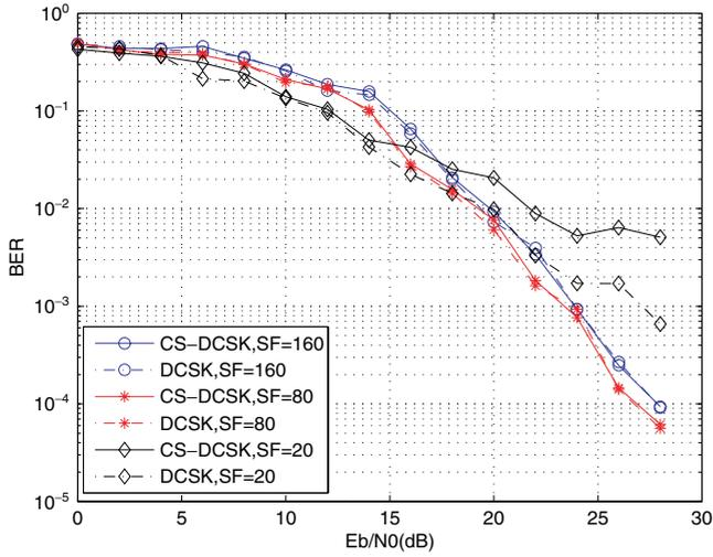
Fig. 13. Performance comparison of CS-DCSK and DCSK modulation schemes over Rayleigh multipath channel defined by model II.
