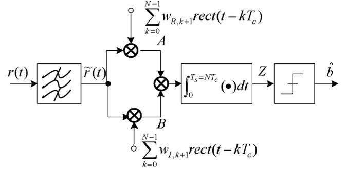
Fig. 4. Block diagram of CS-DCSK receiver.
