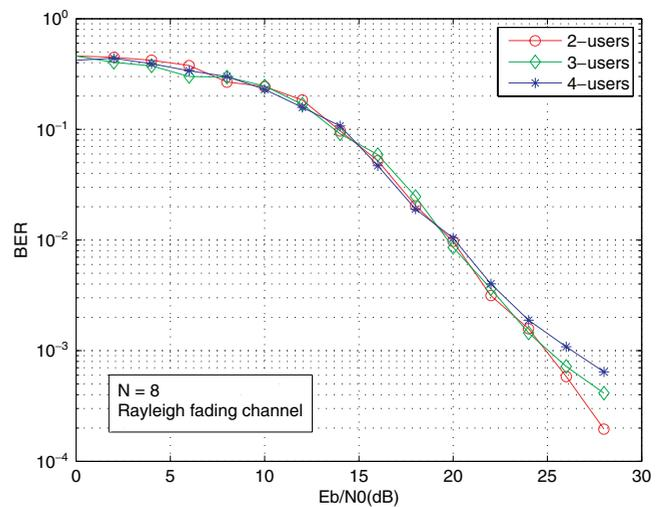
Fig. 16. BER performance of multiuser CS-DCSK over multipath Rayleigh fading channel (channel I), spread-spectrum factor is 160.
