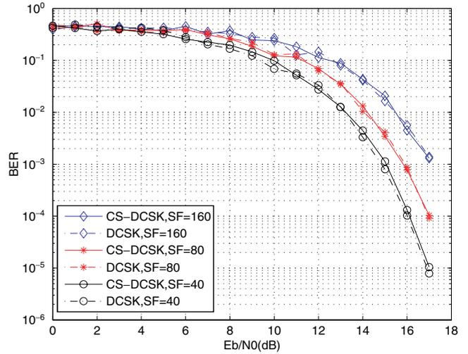
Fig. 11. Performance comparison of CS-DCSK and DCSK modulation schemes over AWGN channels for different spreading factors.
