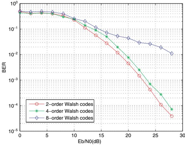
Fig. 10. BER performance of the CS-DCSK modulation scheme in a Rayleigh multipath propagation environment for channel model I. The spreading factor is 80, the parameter is the order of Walsh code.
