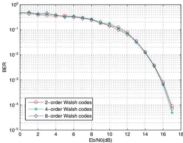
Fig. 7. Effect of the order of Walsh code on the BER performance when the spreading factor is kept constant ( $\omega = N\beta = 80$ ).
