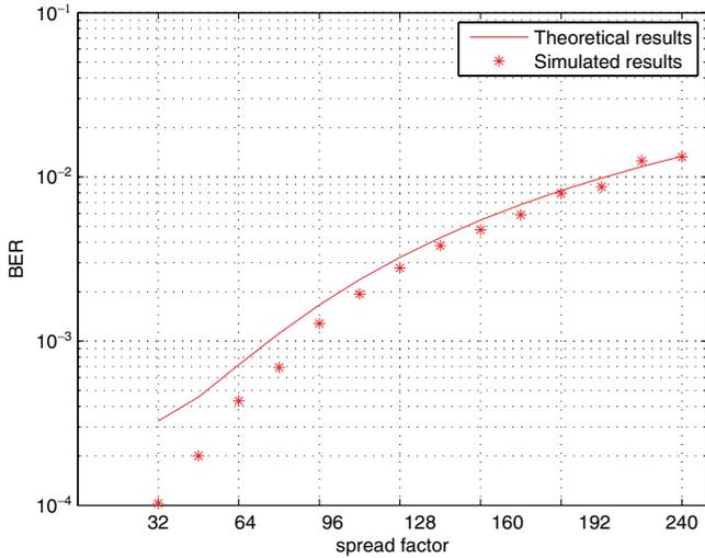
Fig. 6. Effect of spreading factor on BER performance of the CS-DCSK modulation scheme.  $E_b/N_0$  has been fixed at 16 dB.
