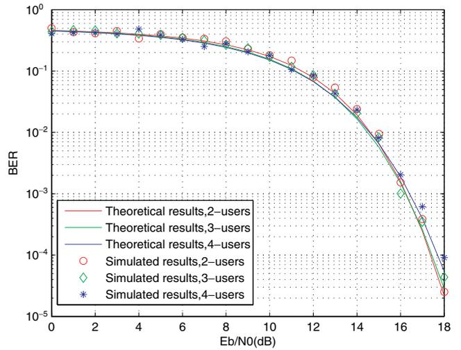
Fig. 15. BER performance of multiuser CS-DCSK over AWGN channel with different number of users for theoretical results (lines), and simulated results (“circle”, “diamond”, and “asterisk”, respectively), spread-spectrum factor is 160.
