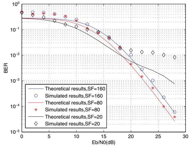
Fig. 8. BER performance of the CS-DCSK modulation scheme in a Rayleigh multipath propagation environment for channel model I. The parameter SF is the spreading factor.
