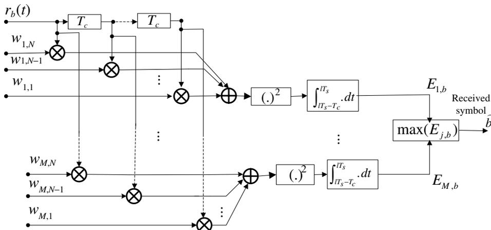
Fig. 2. Receiver of M-ary DCSK based on Walsh code sequences.
