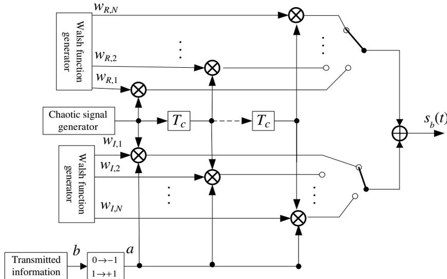
Fig. 3. Block diagram of the CS-DCSK transmitter.
