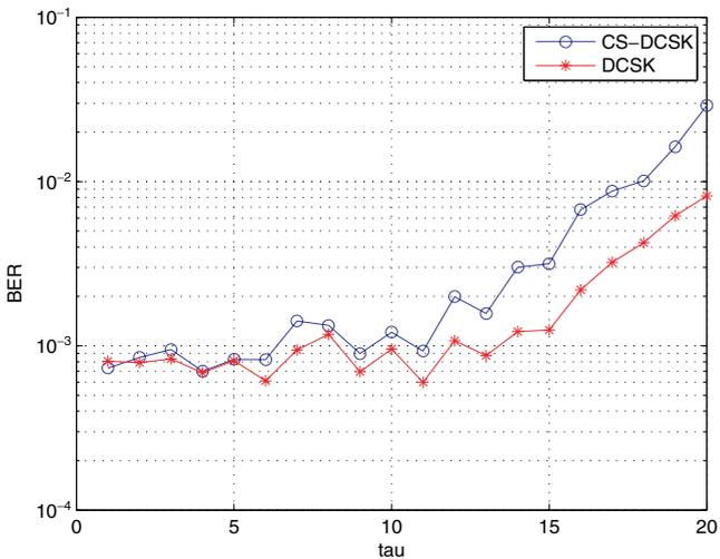
Fig. 14. BER performance comparison of CS-DCSK and DCSK modulation schemes over a two-path multipath channel for  $E_b/N_0 = 26$  dB and  $SF = 80$ .
