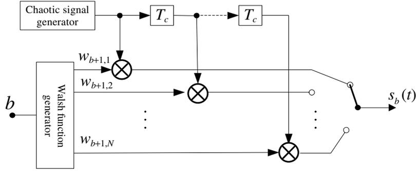
Fig. 1. Transmitter of M-ary DCSK based on Walsh code sequences.
