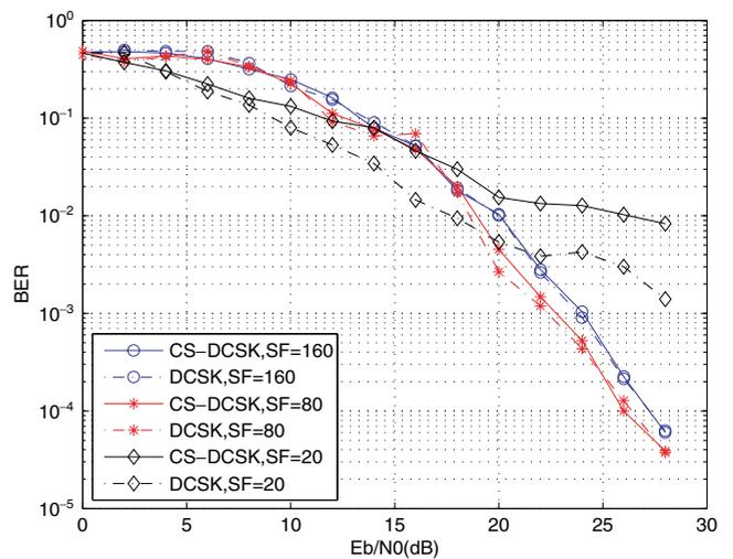
Fig. 12. Performance comparison of CS-DCSK and DCSK modulation schemes over Rayleigh multipath channel for different spreading factors. The channel is defined by model I.
