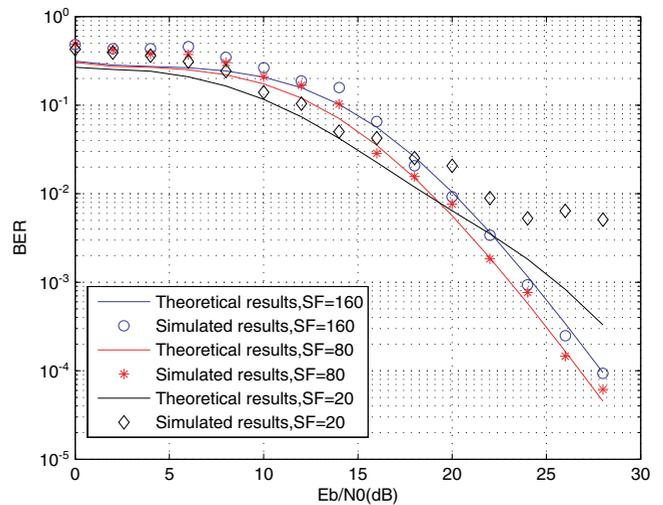
Fig. 9. BER performance of the CS-DCSK modulation scheme in a Rayleigh multipath propagation environment for channel model II.
