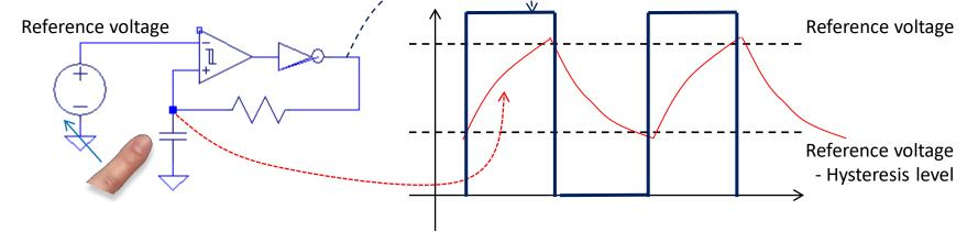
When the finger is close the capacity gets higher->takes more time for charging/discharging->freq. changed->position sensed
