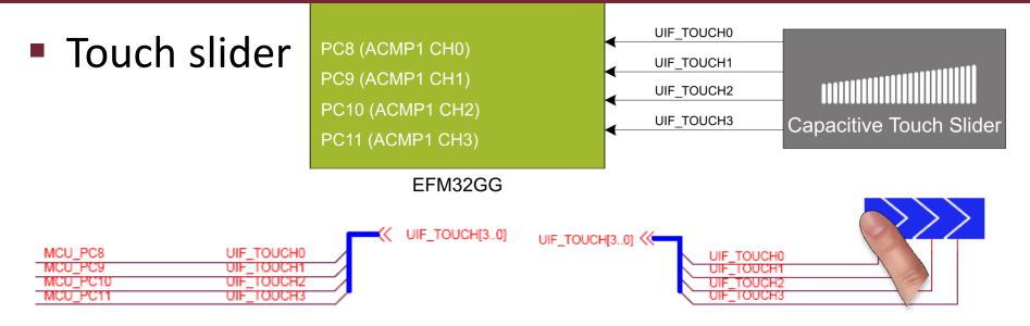
Sensor segments on the PCB. GND layer is not allowed to be placed underneath.
