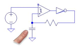
RC oscillator on the PCB. Approaching finger towards copper foil increases its capacity that detunes frequency. The larger the touched area the larger the capacity→ frequency decreased
