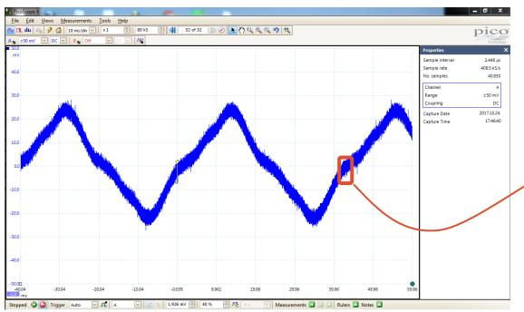
Time function of current signal. Due to the imple implementation the shape is not a sinusoid but a triangle. Frequency is approx. 25 Hz.
