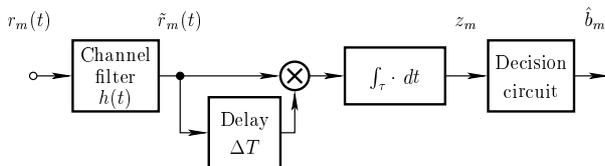
Fig. 3. Block diagram of TR autocorrelation receiver.
