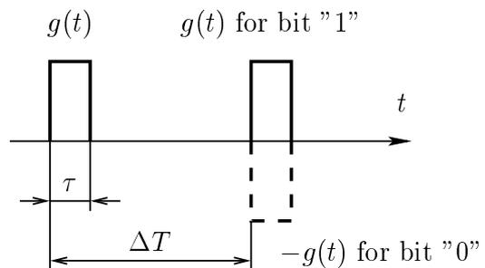
Fig. 2. Structure of generalized TR signal.
