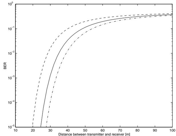
Fig. 4. Noise performance of a UWB FM-DCSK system as a function of distance measured between the transmitter and receiver for different bit durations:  $T = 200$  ns (dashed curve),  $T = 400$  ns (solid curve) and  $T = 600$  ns (dash-dotted curve).
