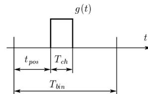
Figure 1: Structure of UWB modulation using one wavelet.
