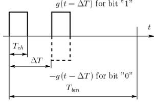
Figure 2: Structure of modulation using two wavelets.
