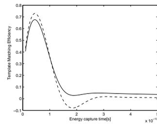
Figure 6: Template matching efficiency as a function of the width of template signal. The RF bandwidths of bell-shaped Gaussian impulses are 2 GHz (dashed curve) and 2.5 GHz (solid curve).
