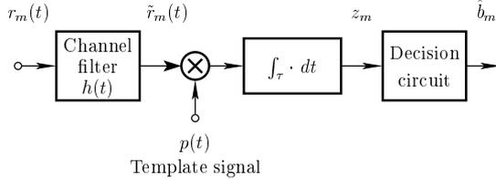
Figure 4: Detection of pulse polarity modulation with a template signal  $p(t)$ .
