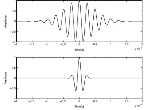
Figure 3: Bell-shaped Gaussian pulse with 500 MHz (upper trace) and 2 GHz (lower trace) RF bandwidths.
