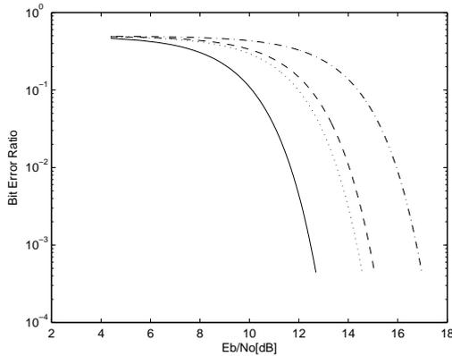
Figure 7: Noise performance of pulse polarity modulation built with template detection. Solid curve: BW=2 GHz and  $e_{tm} = 0.69$ ; dotted curve: BW=2 GHz and  $e_{tm} = 0.40$ ; dashed curve: BW=500 MHz and  $e_{tm} = 0.35$  and dash-dotted curve: BW=500 MHz and  $e_{tm} = 0.20$ .
