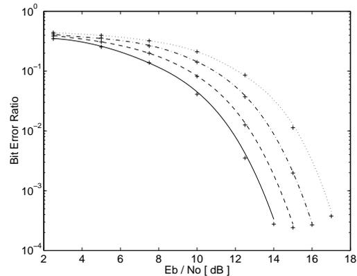
Figure 9: Noise performance of a TR system built with an autocorrelation receiver. From left to right  $2B\tau$  is 8.5, 17, 34 and 68.
