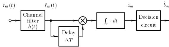
Figure 8: Block diagram of TR autocorrelation receiver.
