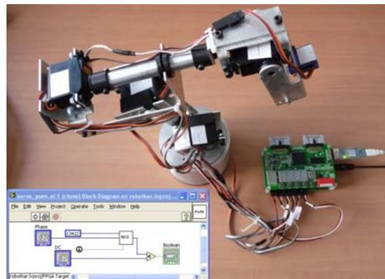
Figure 7. Robot arm control by LabVIEW.
