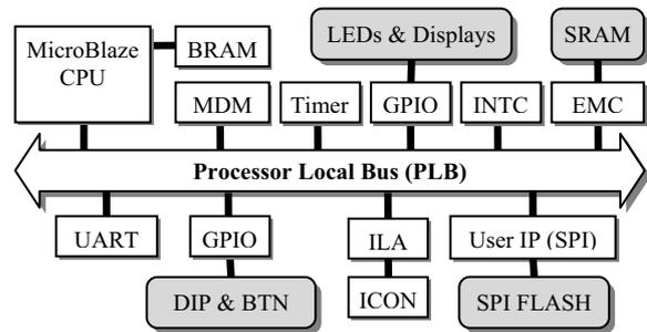
Figure 4. The XUP MicroBlaze reference design
