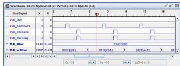
Figure 5. Monitoring PLB on chip bus transfers
