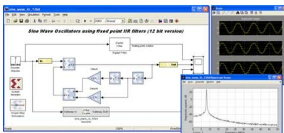
Figure 6. An oscillator using System Generator.
