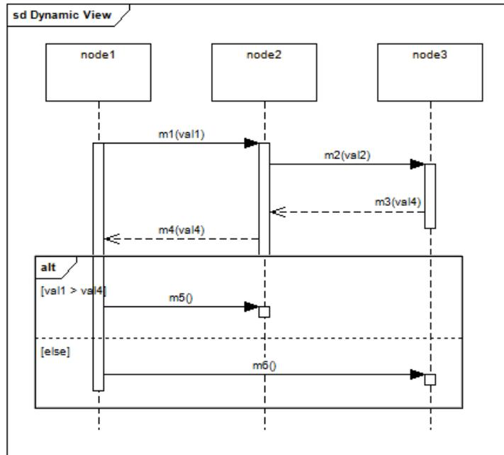
The *Unified Modeling Language 2.0* (UML) [24] is the standard of the Object Management Group (OMG). The language supports behavioural description of applications with *UML Sequence Diagrams*. A diagram represents a single scenario, or as it is called in UML,
