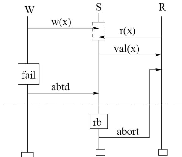
*Triggered Message Sequence Charts* (TMSC) are, therefore, designed to specify such scenarios. A TMSC is constructed of a *trigger* part and an *action* part. The two parts are separated in the diagram by a dashed line. A trigger describes a conditional scenario which may or may not take place during the execution of the implemented system. The
