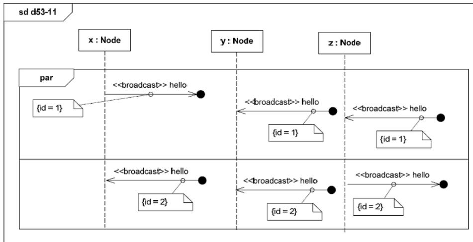
TERMOS event view is also able to handle *broadcast messages*, as it was proposed, specifically, to support the validation of mobile computing systems, among the specificities of which communication with broadcast messages has been identified. The sending of broadcast messages are denoted by UML *lost message* elements (i.e. messages with type
