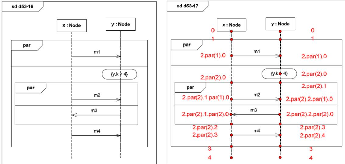
Figure 3.2: A Pre-processed TERMOS Diagram
