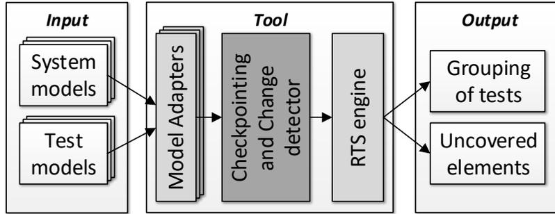
Fig. 4. Architecture and workflow of the prototype tool
