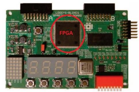
• In this first design, you are going to control the LED panel of the FPGA using the switches: if a switch is turned on, the corresponding LED will light up.
