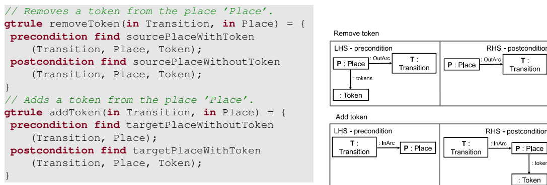
Figure 4: Graph transformation rules for firing a transition
