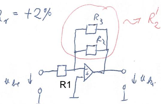
$$R'_2 = R_2 \times R_3 = 5,005 \text{ k}\Omega$$
