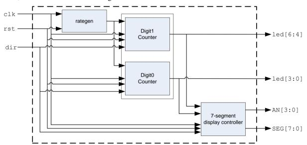
The display consists of 4 digits, each having 7 segments (plus the dot). The display is controlled by 8 segment signals and 4 so-called anode signals – the latter are the enable signals for each digit, as shown below. All signals are active low.
