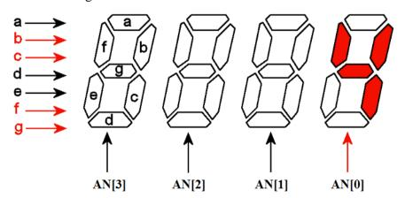
As the segment signals are shared between all 4 digits, the display should be controlled in a time-
