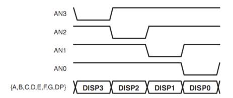
Circulating between the 4 digits should be slow enough to have enough time to turn on the LEDs, but should be fast enough for the human eye not to see blinking – the appropriate frequency is in the kHz range.
