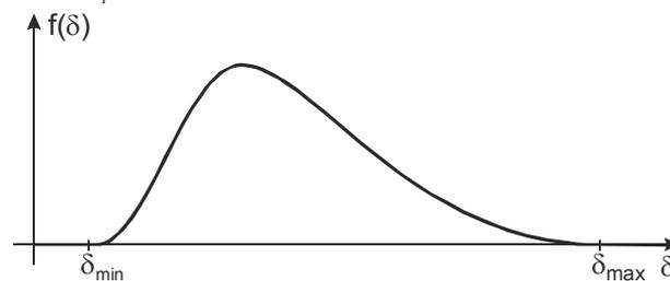
Figure 1 – Distribution function of the delay  $\delta$
