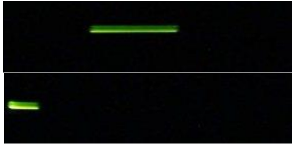
Fig. 12. Blur of the active marker at around 200 rpm (3.24 Hz), T_v=1/30 s, ISO 6400, two different samples. Width of the picture corresponds approximately to the range of the movement, i.e. the trail corresponds to \sim 10\% of one circle.
