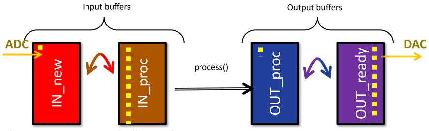
After processing interchange of buffers is performed (status after interchange is seen)
