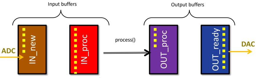
Data is continuously arriving into one of the input buffers from ADC while the content of the other buffer that is full is being processed Processed data is continuously arriving into one of the output buffers while the content of the other buffer that is full is being sent toward the DAC
