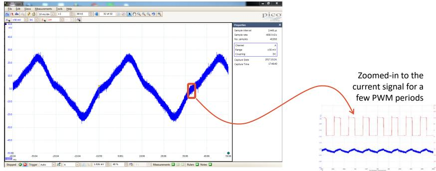
Time function of current signal. Due to the imple implementation the shape is not a sinusoid but a triangle. Frequency is approx. 25 Hz.
