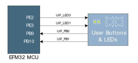
PB0=push button nr. 0 PB9=9<sup>th</sup> bit of port B PE3=3<sup>rd</sup> bit of port E
