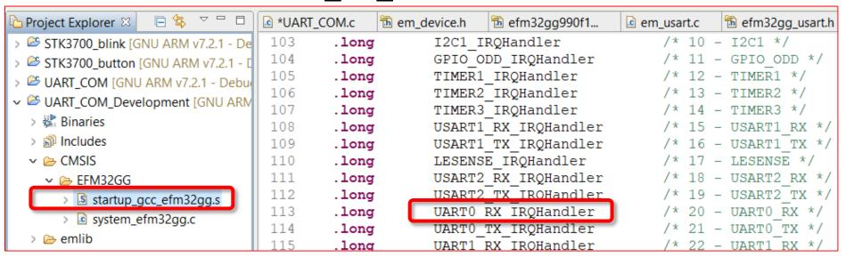
UARTO\_RX\_IRQHandler is a weak function so it can be overdefined in the program without causing any error:
