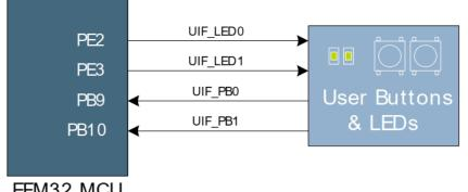
PB0=push button nr. 0 PB9=9<sup>th</sup> bit of port B PE3=3<sup>rd</sup> bit of port E
