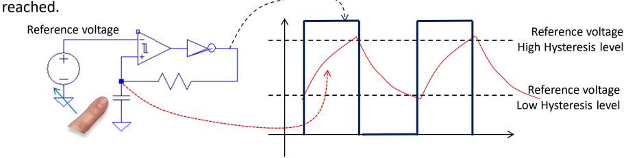
When the finger is close the capacity gets higher->takes more time for charging/discharging->freq. changed->position sensed
