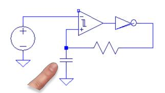
RC oscillator on the PCB.
