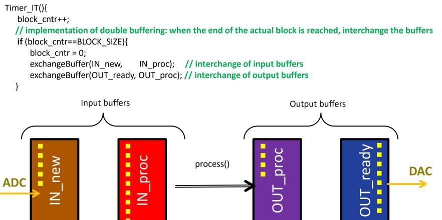
Data is continuously arriving into one of the input buffers from ADC while the content of the other buffer that is full is being processed
