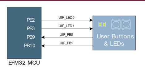
PB0=push button nr. 0 PB9=9<sup>th</sup> bit of port B PE3=3<sup>rd</sup> bit of port E
