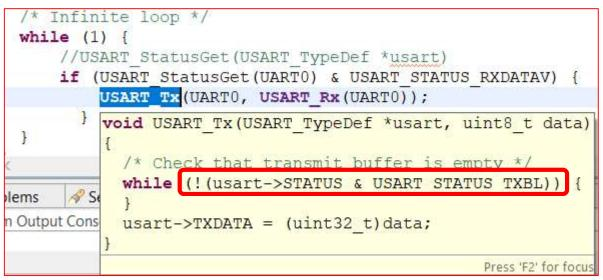
Clearly seen that blocking may happen but "less severe" -> USART\_STATUS\_TXBL bit is checked in STATUS register
