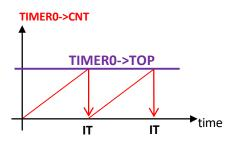
In simple timer mode of the Timer, the value of the CNT register increases by one for each cycle of the input clock until the value stored in the TOP register is reached. Then the CNT counter resets and generates an interrupt on the corresponding interrupt line (TIMER\_IF\_OF).
