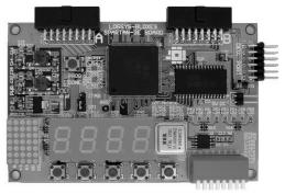
Figure 2 The LOGSYS Spartan-3E FPGA board.
