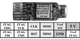
Figure 1 The LOGSYS development cable.
